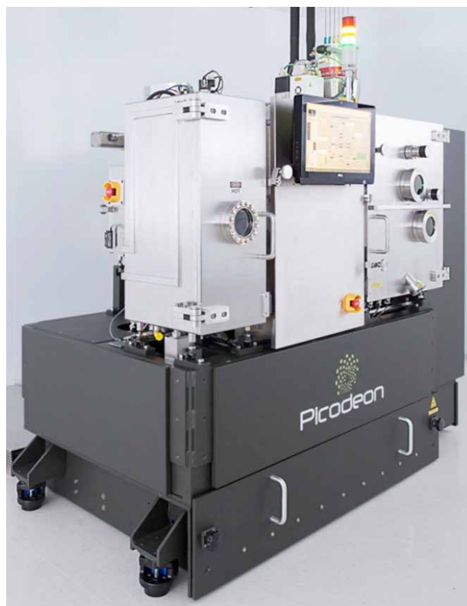
Picodeon Series4 semi-industrial automated PLD system
