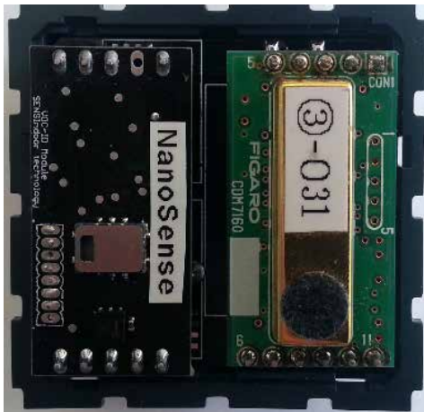
Fig. 2b: Field test electronics demonstrator (NanoSense) sensor module aside an NDIR CO 2 module
