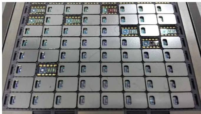
Fig. 4: Array of assembled and capped \mu\text{PC} +sensor systems. On the samples without cap, the \mu\text{PC} and a dual MOS sensor are visible (close-up view in Fig. 5).
