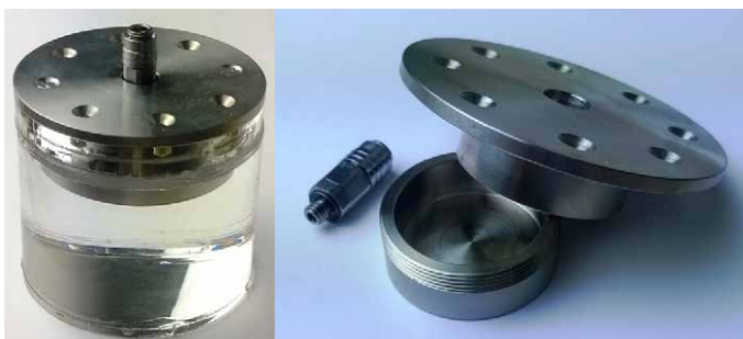
Fig. 3: Calibration standard with (left) and without (right) phase change material cladding.
