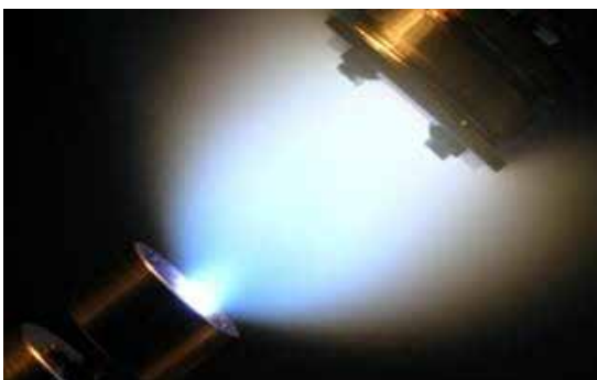
Fig. 1 a) Bluish plasma plume generated in the PLD process, and b) a schematic of a typical PLD system
